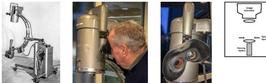
Another variant of a single channel system is shown in Fig 30. Figure 30 illustrates a c 1955 table mounted gantry equipped with monocular viewing, a photographic camera that could be placed into the single viewing channel. The operator could not see the images while filming. Its optics are shown schematically for fluoroscopy and fluorography.
