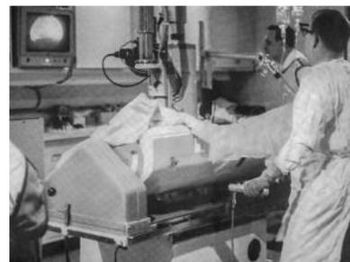
Gantries with one and two degrees of rotational freedom were introduced in the 1970s (Figure 40). Moving gantries were safer for patients but needed new forms of staff scatter protection to replace that provided by fixed X-Ray tubes located in a shielded table base. Simultaneously optimizing patient safety, physician-patient access, and staff safety is still evolving. There is an extensive literature on this topic. A small subset is referenced in this paper<sup>24-41</sup>.
