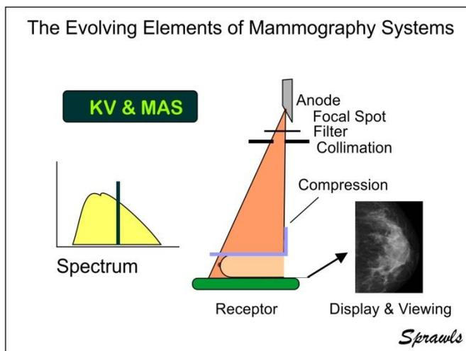
Figure 2. The elements of the mammography system that have evolved over the years in the effort to provide better visualization within the breast.
