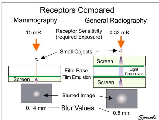
Figure 21. Comparison of intensifying screen receptors for mammography to general radiography.
