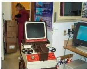
b) Cine film viewer. The boxes in the background are part of the daily image transfer between the lab and its off-site archive. Each box contains 50 rolls of cinefilm. Image storage and retrieval was on a 24-hour cycle.
