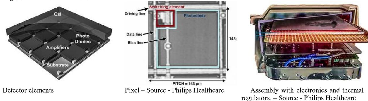
FPS reduce or eliminate several inherent image-intensifier artifacts. These include vignetting (images dimmer in the periphery relative to the center), pincushion-distortion (result of projecting a curved input screen onto a flat output screen), S-distortion (electro-magnetic field influence on the II’s electron optics), and II dynamic range limitations.
