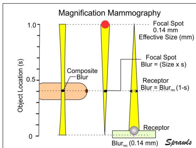
Figure 27. The use of geometric magnification to reduce the effective receptor blurring and increase visibility of small calcifications.
