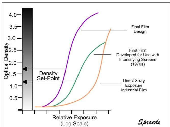
Figure 14. Characteristic (H & D) curves of the three major phases of film used for mammography.
