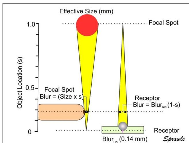
Figure 25. The effect of breast location (“s” scale) between the receptor and focal spot on the blur from those two sources.
