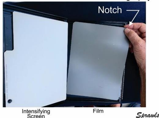
Figure 22, Inserting film into a single screen mammography cassette. This was in a darkroom so there was a notch in the film to identify the upper right corner when viewing the emulsion side.
