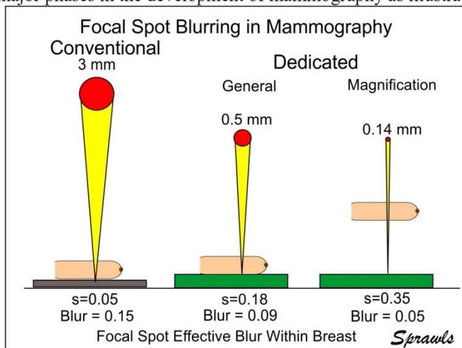
Figure 26. Three focal spot sizes that have been used in mammography.
