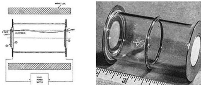
**Fig 25: Image intensifier with minification**
