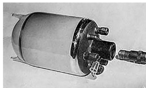
With image intensifiers, dark adaptation and dark fluoroscopic rooms were no longer required. Early image intensifiers had brightness gains of a few hundred times that of the brightness of the input screen. To permit operation at normal room
