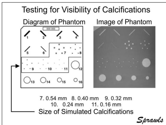
Figure 24. Diagram and image of the breast phantom that became a standard for evaluating mammography equipment performance.
