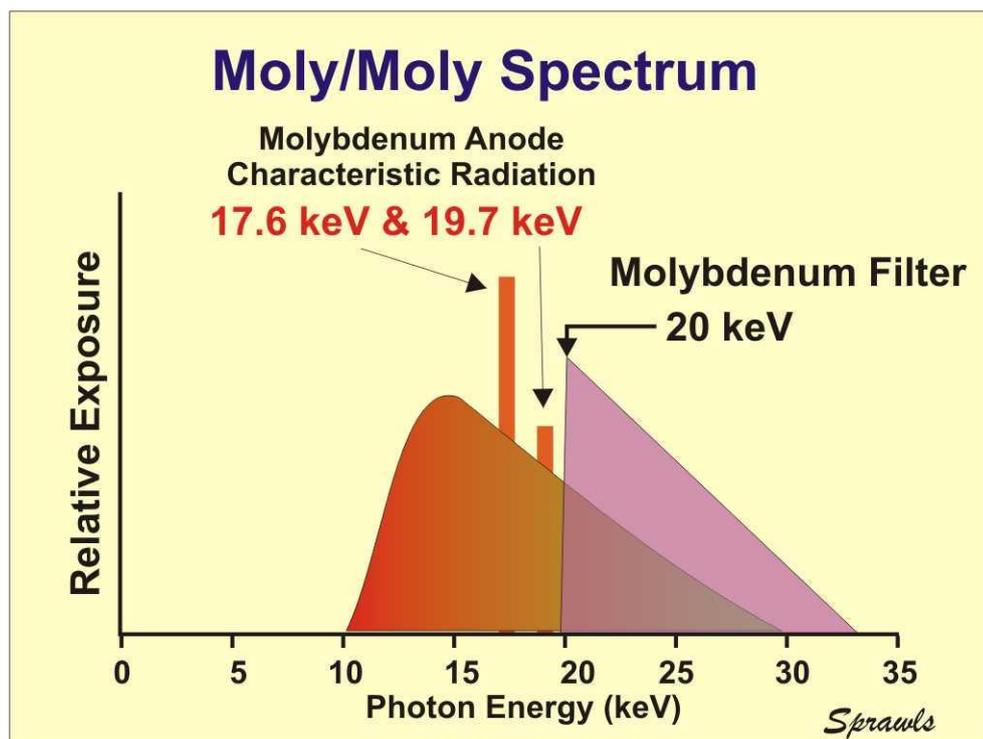
Figure 10. The x-ray spectrum produced with the combination of a molybdenum anode and filter.
