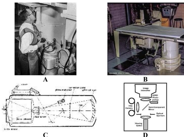
As noted above, this 11-inch device includes a photo pickup which indicates that the fluoroscopic system included an Automatic Brightness Control (ABC) circuit. Because such circuits work by controlling radiation output, the nomenclature changed to Automatic Dose Rate Control (ADRC). Photo pickups were incorporated into the optics used for most of the systems incorporating analog video chains. Further examples are shown in the sketches of image intensifier optics presented later in this paper.
