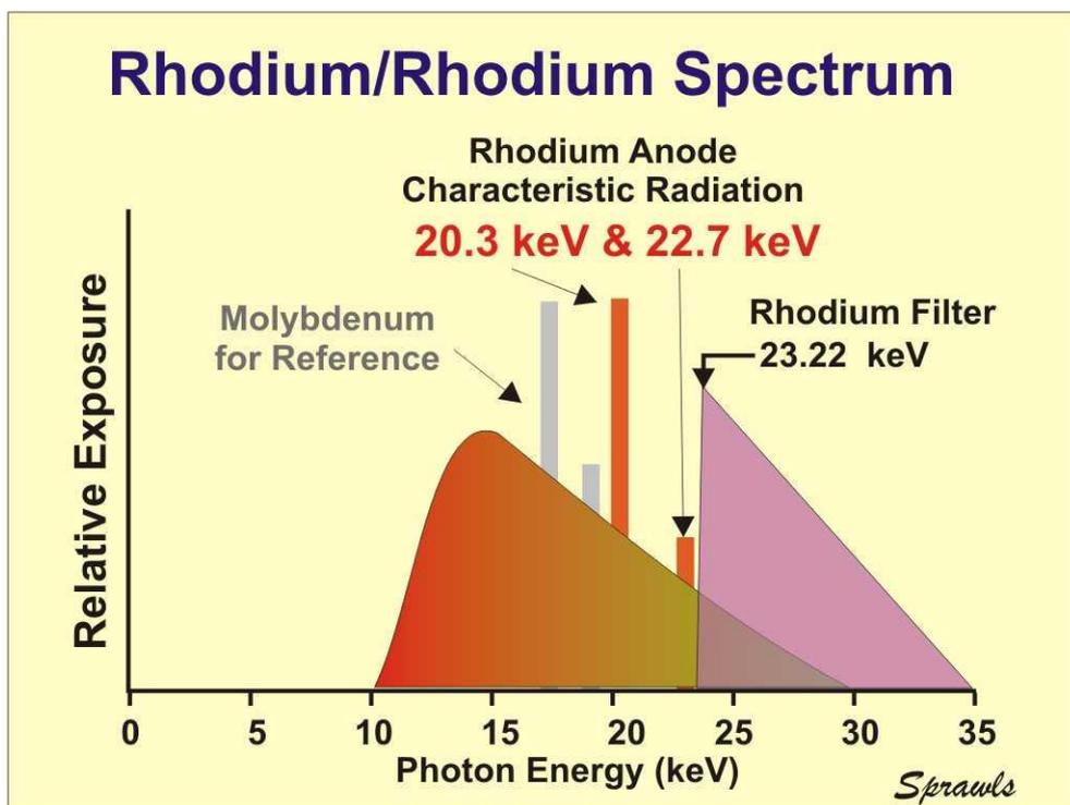
Figure 11. The spectrum produced with a rhodium anode and filter.
