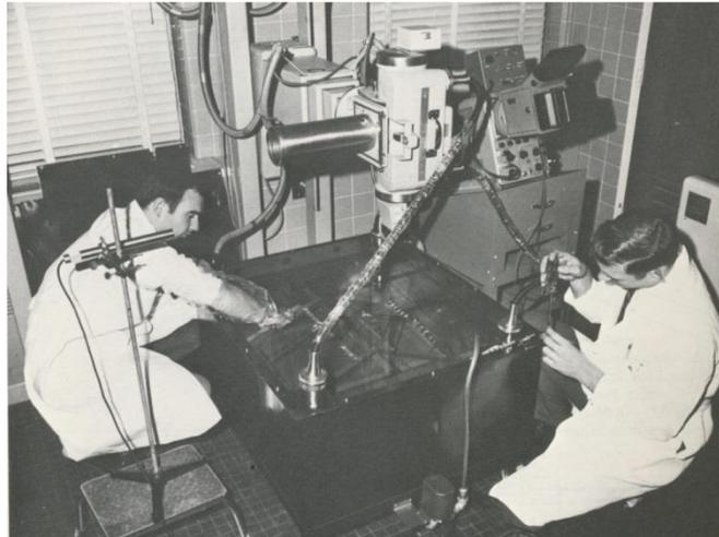
Figure 9. Physicists using a bank of resistors in a tank of insulating oil as an electrical load to evaluate the performance of x-ray generators being developed for mammography
