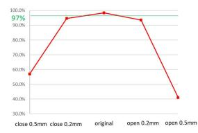
*Figure 3 Passing rates using the gamma index 2%/0.5 mm criteria for MLC error types.*
