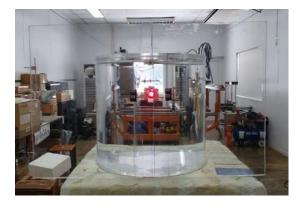
*Figure 2* Setting up nanoDot dosimeters on the PMMA water-filled cylindrical phantom with solid PMMA slabs.
