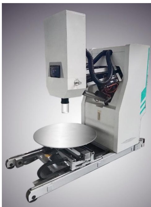
Fig. 1 The domestically developed intraoperative radiation therapy (IORT) robot prototype.
