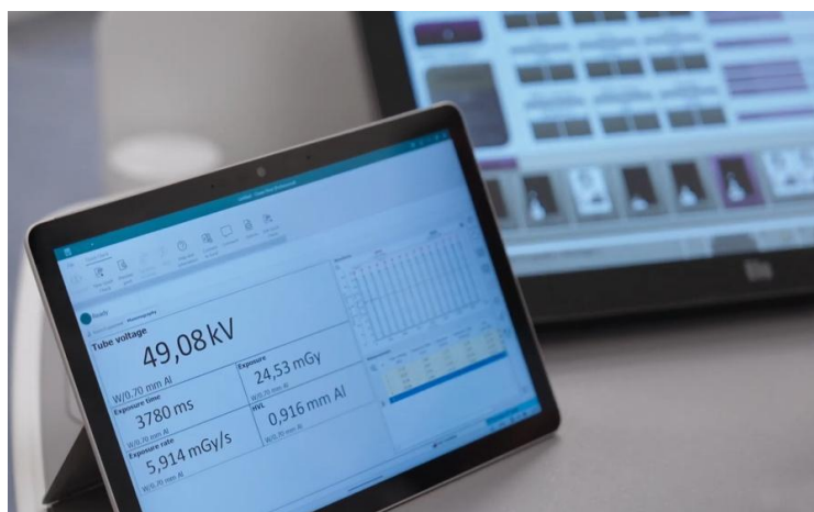
Picture 1. With the Ocean computer software all measured parameters can be seen at the same time, including waveform.
